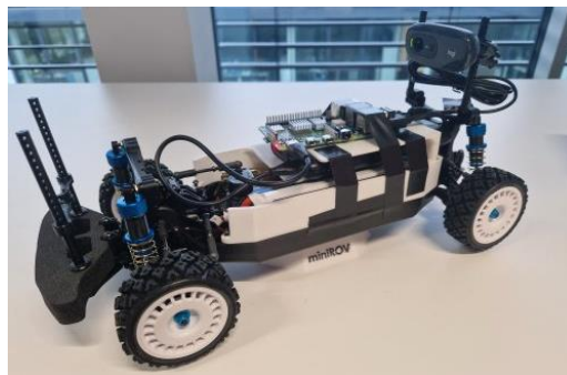
Figure 1: The current proto-miniROV, based on an RC-car frame.
