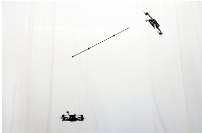
Fig. 1. Illustration of two quadrocopters passing a pole between them. The right quadrocopter throws the pole towards the left vehicle, which tries to catch and re-balance it.
